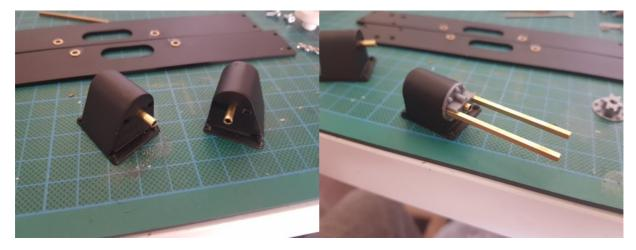
Take the 2 cross-heads and glue in the 2mm steel rod next fit the cylinder to the chassis with 2 3mm x 8 cab head bolts slide the cross-head in to the tube then fit the slider bar holder test the cross-head must move freely once happy it moves freely add a dab of glue to the slide bar holder and use super glue on the rear cylinder cover and slide bars leave to dry.
