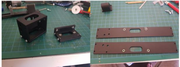
DO NOT GLUE AT THIS TIME. next take the cylinders push in the 3mm x 20mm brass tube must have about 7mm sticking out you will see that there 2 sq holes in the rear of the cylinder push in the 2 sq brass rods and the rear cylinder cover
