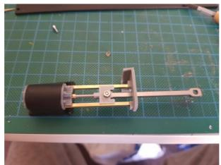
next take the gearbox housing and drill the bearing holes to 4mm push in the axle then fit the bearing making sure it turns freely when happy add a dab of glue to the bearing to hold in place. Next fit the worm to the motor leaving a cap of about 1.5mm using 2 3mm x 6mm long bolt the motor to the gearbox housing make sure you have the meshing right test the motor on a 3 volt battery when happy add some oil to the gears.
