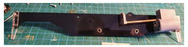
There are 2 frame spacers, 1 L shape (front) and one U shape (rear). Using 4 x 2mm x 10mm bolts and 3 x 2mm x 8mm bolts these can now be fitted to the left hand frame.
