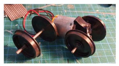
The wheelsets can now be fitted to the frame with the frame spacers attached. Start by pushing the front axle through the front bearing in the frame, the gearbox should be fitted with the 'bulge' facing
