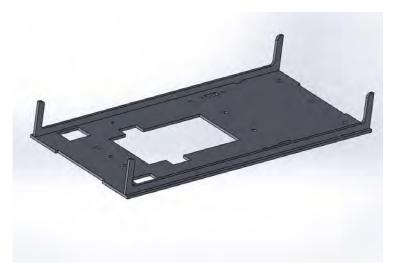
Next glue the buffer beam inner onto either end to strengthen the ends. Now the buffer beams can be glued onto either end, a screw through the coupling hole aids alignment.
