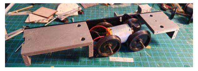
The right hand frame can now be fitted using 4 x 2mm x 10mm bolts and 3 2mm x 8mm bolts.
