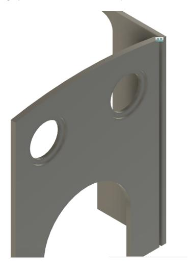
34. Once the sides and front have dried attach the back panel making sure the sides locate properly on the rear cab sheet as pictured. Then glue and let it dry. Once dry
