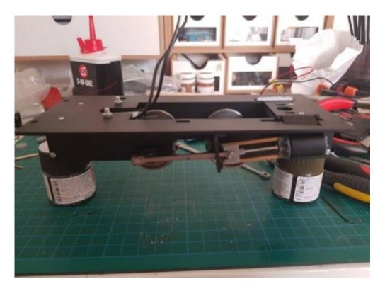
28. Once you have a smooth-running chassis it is time to fit the foot plate. This comes as a single piece of laser cut acrylic. You will need to countersink the 4 holes to take
